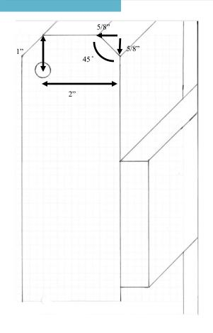
Measure from the bottom of each leg on the furthest face from hole drilled in the step above and notch out a 31/2" by 3/4" housing for the leg rails.
