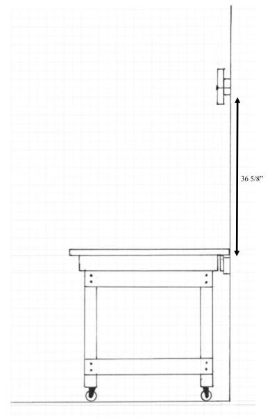
Note: To protect the bench, some form of matting for example thin pin board material can be mounted on the wall between the bench top and the wall.
