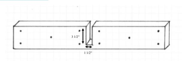
Take spreader bar housing rail (3  $1/2 \times 3/4$ " x 22 3/8") measure and mark centre. Centring over this point mark 1 1/2" x 3 1/2" housing to take spreader bar.
