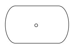
On the smaller locking mechanism timber (3 1/2" x 3 1/2" x 8"), mark centre and drill through with 3/8" hole.
