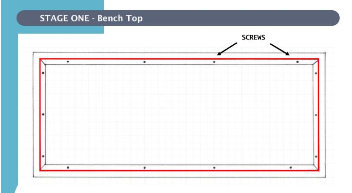
Starting with the bench top (83"(L) x 36"(W) x 1 1/2"(T)) laying face down, mark a 2 11/16" border around all edges. This marks the outside of the apron.
