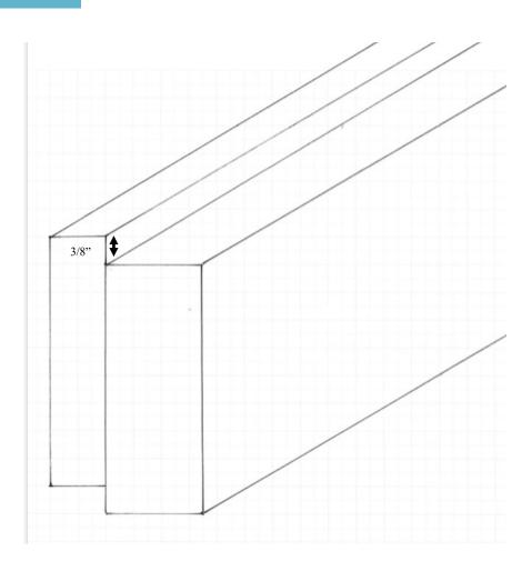
Take your 3 1/2" x 3/4" x 16" support rail timber and attach it to the 3 1/2" x 2 1/2" x 16" support rail timber leaving a 3/8" lip using 8 evenly spaced 2" timber screws.
